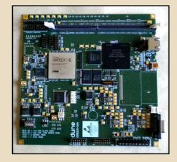
The board can be employed as a versatile test bed for a radar receiver or a SDR (Software Designed Radio) communication receiver; the high data rate of its ADC is suitable to process wideband signals or to implement sub-sampling techniques.
