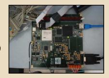
Connection FPGA-external computer by a fast connection (Gbit Ethernet).
