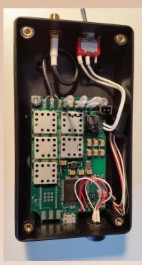
The system includes an Inertial Sensing Unit to be attached inside or outside a shoe heel, a Computing Unit processing raw data and a MMI SW used to acquire, integrate and display the path walked by the operators wearing the system.
