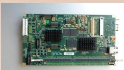
All-purpose FPGA VIRTEX 5, 6 and 7 Platforms and a Freescale communication processor
