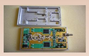
RF Demodulator 400 MHz – 5 GHz Large Band I/Q conversion in base band
